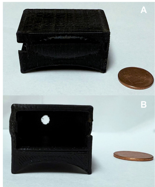
Figure 1. Lateral view of 3D printed GPS logger harness. Anterior view of 3D printed GPS logger harness. American penny (1¢) used for scale. Photo by Jordan Donini.
